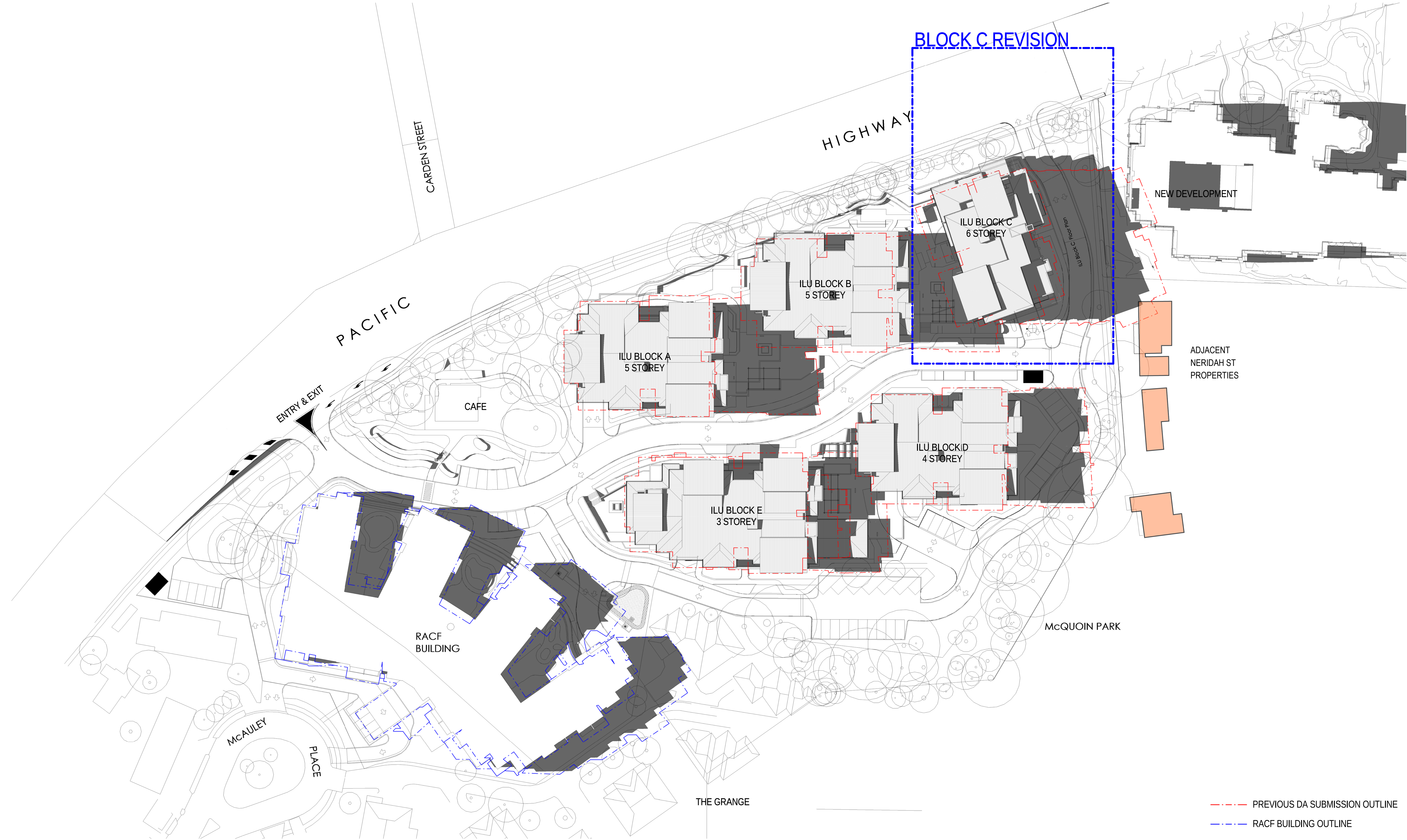
1 21 JUNE 12NOON - SHADOW DIAGRAM PLAN VIEW SCALE 1 : 400
