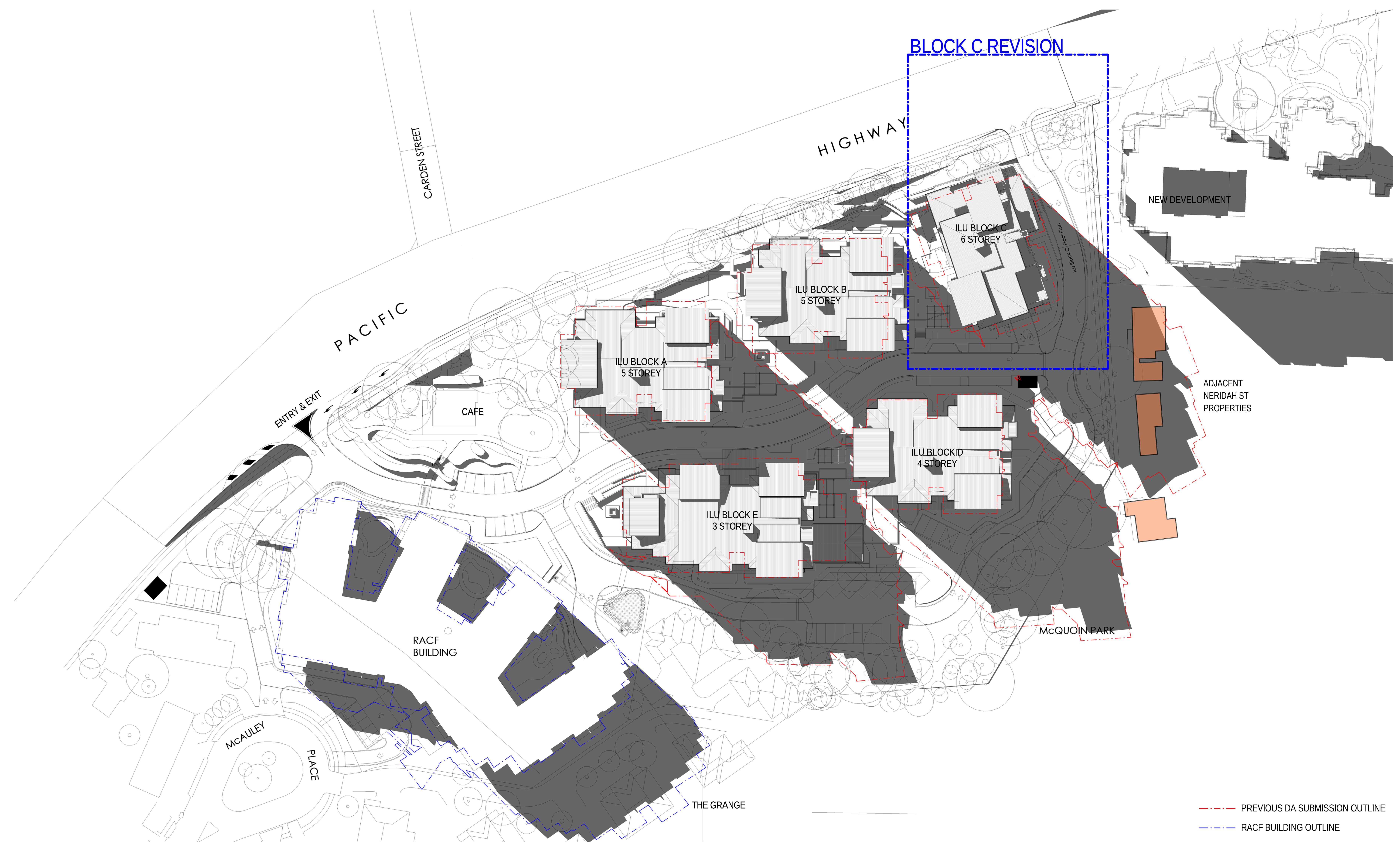
1 21 JUNE 9AM - SHADOW DIAGRAM PLAN VIEW SCALE 1:400
